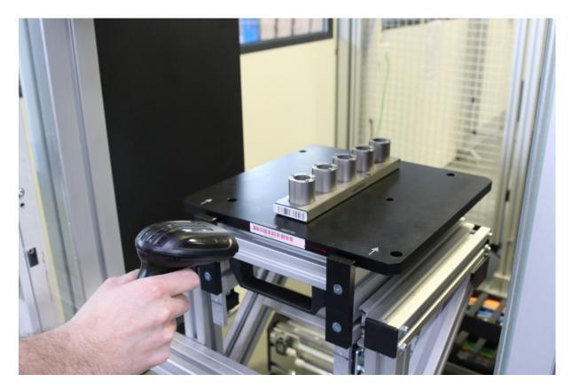
After logging on to the central computer of the system using a personalised data chip or password, the operator scans the barcode printed on the order card, places the pallet in the I/O station of the cell and registers the order with the system by scanning the pallet barcode. The robot transports the pallet to one of the 50 rack positions in the cell and feeds the two coordinate measuring machines alternately with the orders that are further along in the sequence.
