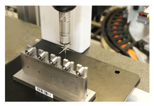
Consequently, KOMEG's concept included two "574s", each equipped with two probe change racks which are alternatingly loaded by robots. The custom solution also includes a shelving system in which up to 50 pallets with clamping devices and workpieces can be stored until they are inspected.
