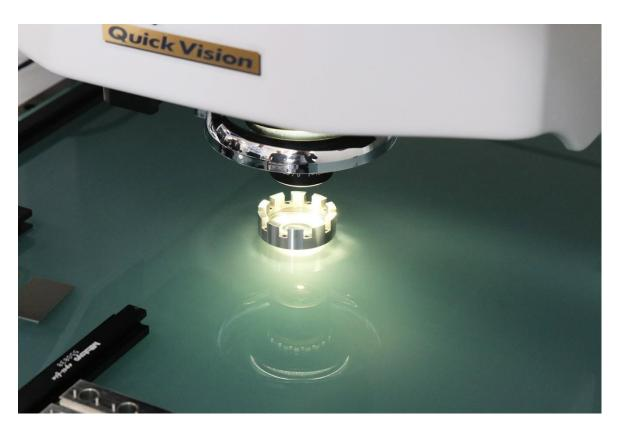
And with the Mitutoyo measuring machine, GFH kills three birds with one stone. Due to its measuring uncertainty of only 0.25  $\mu$ m, the 3D CNC vision measuring machine is perfectly suited for the calibration or compensation of their own machines. Thus, it can measure circular-lasered test workpieces with an accuracy of up to one micrometre.
